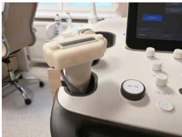
Figure 1. A 3D-printed cover for the ultrasound probe that was used to measure the mechanical pressure exerted by the probe during an elastographic examination
