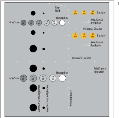
Figure 1. Scheme of the phantom used for evaluation of ultrasound scanners (source: [20]). During measurements, the transducer is in contact with the top surface of the phantom.
